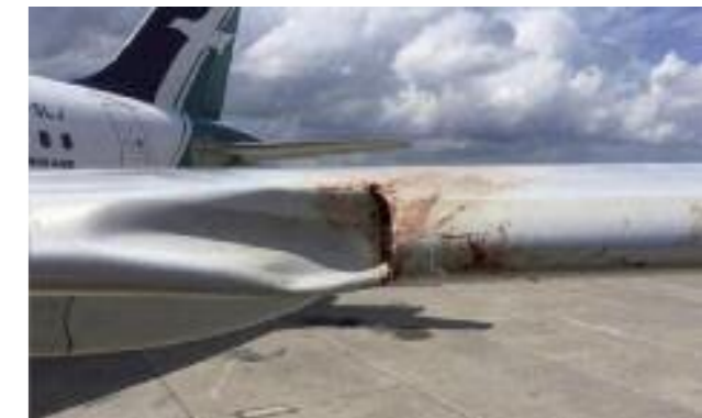
Damage to an A320 after a bird strike, 2015
